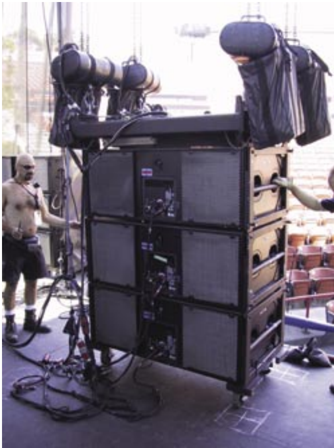
Figure 31. Fully rigged M3D block ready to fly
